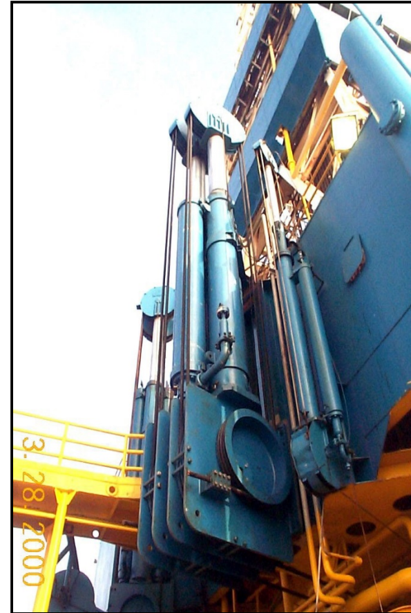
160 Kip Ram Tensioners on Drill Rig
